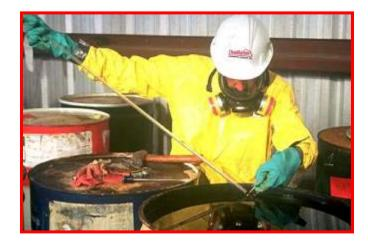
The Lambton Acid & Alkali Plant receives liquid wastes for neutralization. The wastes are blended in a controlled neutralization process and fed to the incinerator for final processing. The pretreatment process features large throughput and has the capability to receive waste in bulk, drums and totes.
